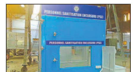
On entering the chamber, an electrically-operated pump creates a disinfectant mist of hypo sodium chloride for disinfecting ANI
